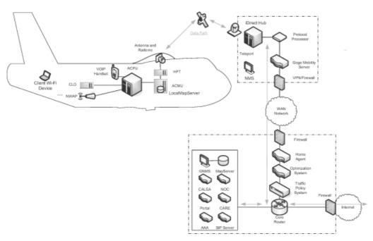
The data rates available to an aircraft using Ku-band or Ka-band satellite technology will vary based on a number of factors such as the satellite used, its coverage area and specifications, the aircraft location, aircraft antenna and modem capabilities. We expect the peak data rates to be approximately 40 to 50 Mbps to an aircraft and approximately 1 to 4 Mbps from an aircraft.
